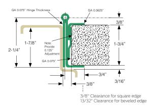
\* Adjusta-Stud allows up to 3/6" width adjustment which ensures proper alignment and easy installation. Adjusta-Stud also makes it possible for future adjustments of the door on the frame through repositioning. If using Adjusta-Stud, 14 gauge reinforcements on frame and door required.
